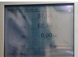
62.5% methane in total generated biogas
